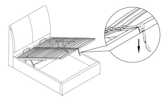
Lift with the strap (16) and close as per guidance on page 7. The strap should always be accessible. Take care not to lean over the bed when lifting, if the mattress is thin and light, the frame may rise quickly. The speed of closing will also depend on the weight of the mattress so always keep fingers well clear of the metal frame.
