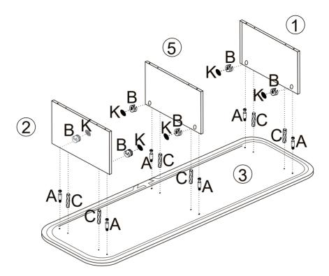
STEP 2: Insert the back panel(6) with side panel (1),(2).
