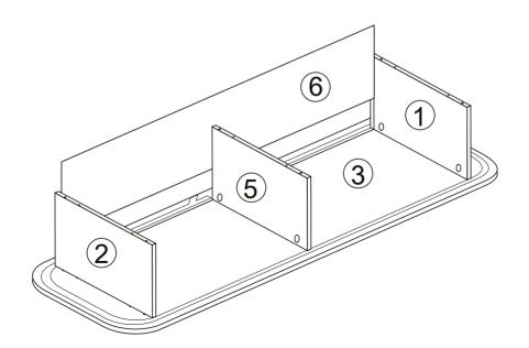
STEP 3: Attach the bottom panel(4) with side panels(1),(2),(5) by hardware (C,J,L);
