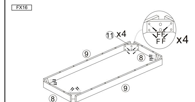
STEP 6: Attach the frame with bottom panel (4) by hardware (C,T).
