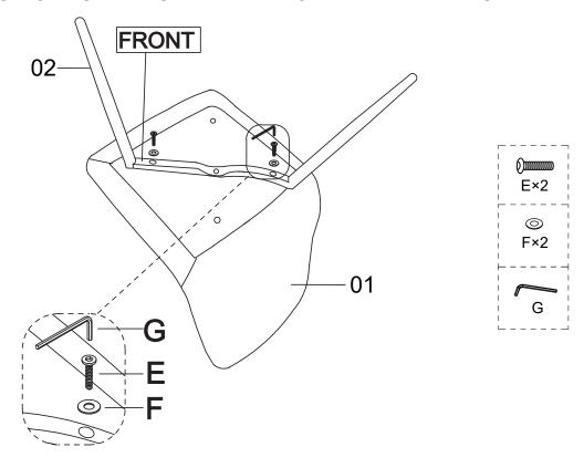
Step 2:Please attach the Leg(03) with the Seat(01) by hardware D,E,F. ATTENTION:DO NOT FULLY TIGHTEN THE BOLTS AT THIS STAGE!
