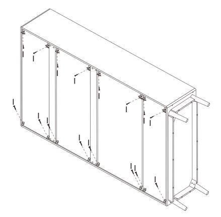
Step 11: Attach hardware T on door(12),(17) by hardware U; Then, attach the handle H and the hardware S. DO NOT use any power tools as this may damage the frame and will invalidate any claim.
