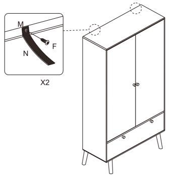
PLEASE NOTE that wall fixings are not supplied as different wall materials require different fixing devices. You must use fixings devices suitable for the type of wall you intend to mount product to. Ensure the head of any screw used has a diameter greater than the mounting hole and the fixing is safe and secure before use.
