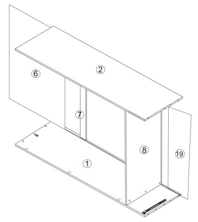
Step 7: Attach hardware A on top panel(3); Then, attach hardware(R) on top panel(3). Attach the top panel (3) with frame by hardware B,C,K.
