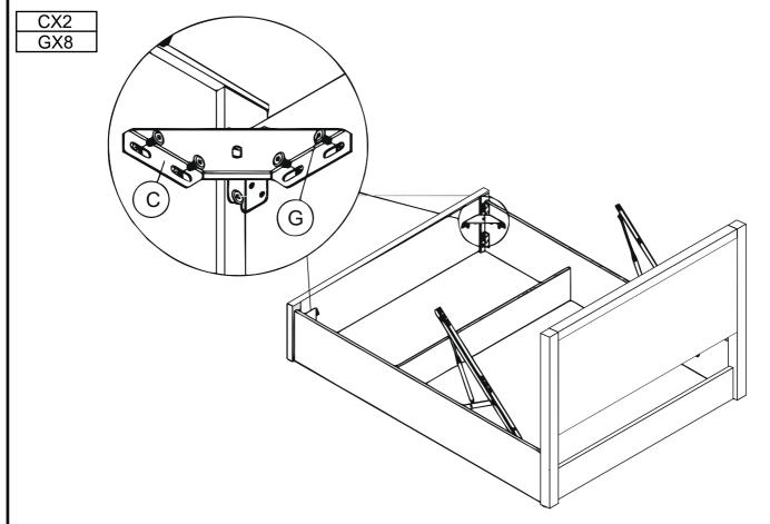
Step 5: Join together all the bed base parts (11),(12),(13) and (14) using hardware parts S,X & R and also slide part P onto Part 14 before bolting together. Attach the centre rail(15) with Metal Frame by hardware G,X&R.And then attach hardware parts J as shown.
