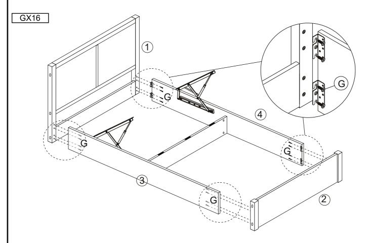
Step 4: Fix the Metal Corner Block(C) by Hardware(G).
