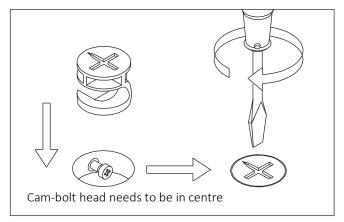
Use a Flat Screwdriver or Phillips Screwdriver to turn the Cam-lock clockwise one half a turn so it locks onto the head of the Cam-lock. Turn only until it is snug. Over-tightening could damage Cam-lock or/and Cambolt.
