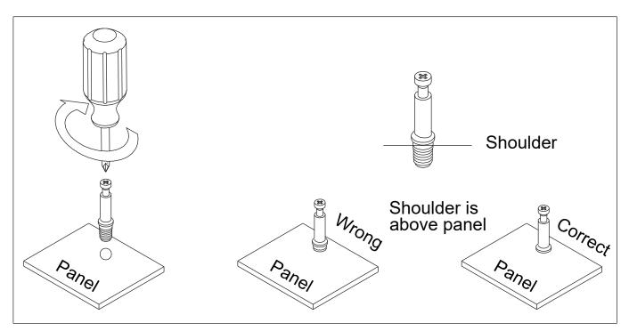
Attach the Cam-bolt to the specific pre-drilled holes on the panel. Use a Phillips Screwdriver to tighten Cam-bolt vertically until shoulder is flush (on the same level) with panel. Do not over-tighten or under-tighten.
