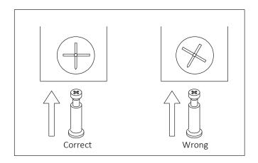
Align the arrow of the Cam-lock to the Cam-bolt head and insert the Cam-lock.
