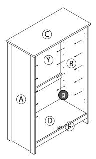
NOTE: The side panel has an extra hole to insert a shelf support, shelves can be adjust to a 15 degree angle or be fitted horizontal.
