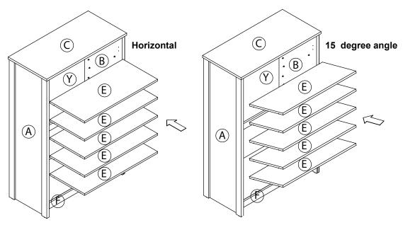
NOTE: Please insert the shelves at a 15 degree angle or horizontal before fitting the doors.
