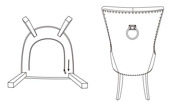
IMPORTANT Carefully turn the chair upright and place on a flat surface. Make adjustments to ensure that the chair frame is straight and that the legs are even on the floor then FULLY TIGHTEN ALL BOLTS assembled in previous steps using Allen key (C).
