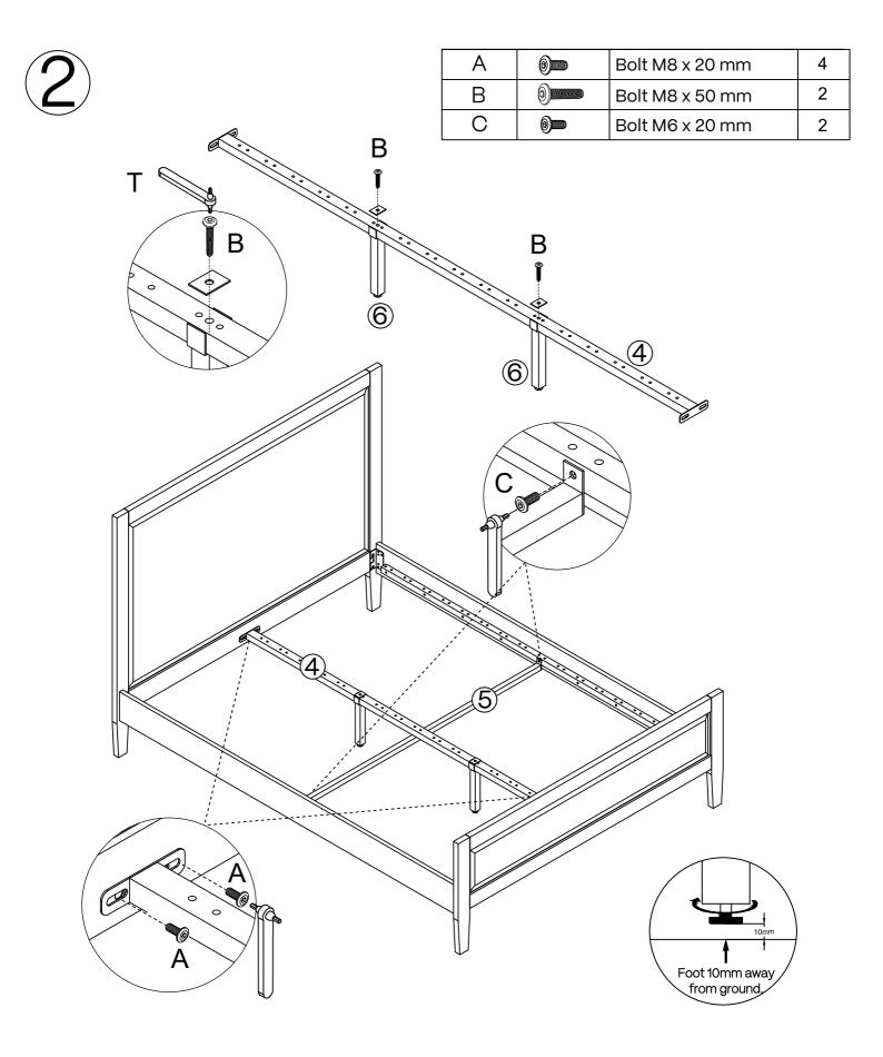
ATTENTION: After central rail and support legs have been assembled, rotate adjustable feet to make support legs 10mm away from the floor. Support legs would touch the floor when a mattress is put on the base.
