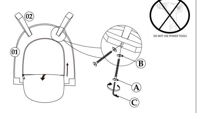
Please do not fully tighten any bolts until the final step.
