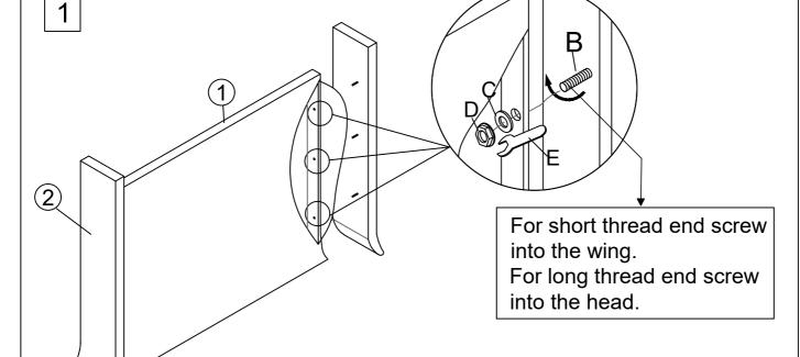
Turn the top of Headboard(1)&Wings(2) upside down on the ground.Attach the Lead screw(B) into the Wings(2) firstly. Then mount both Wings(2) to Headboard(1) by pushing the Washer(C) and Hex Nut(D) to fit . Tighten Hex Nut(D) with Solid Wrench(E).
