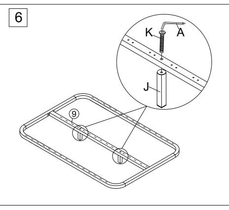
Use Allen Key(A) To fix the Central Legs(J) under the Metal Central Beam(9) with Bolts(K).
