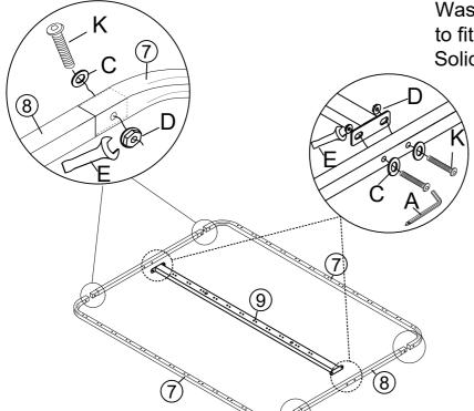
Use Allen Key(A) To attach the Metal Central Beam(9) with Bolt (K) by pushing the Washer(C) and Hex Nut(D) to fit. Tighten Hex Nut(D) with Solid Wrench(E).
