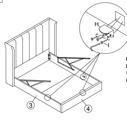
Use Allen Key(A) to Fix the Plastic Support (H) onto the Siderails(3) and Footboard (4) with Screws (I)
