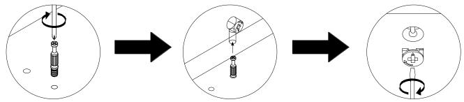
STEP 1 - USE A CROSS SLOT SCREWDRIVER TO TIGHTEN THE CAM BOLT INTO THE HOLE.
