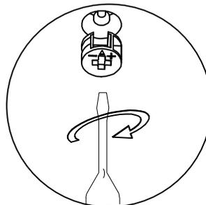
**STEP 3 - THE HEAD OF THE BOLT GOES INTO THE WIDE MOUTH OF THE CAM LOCK. YOU THEN TURN THE LOCK SO THE NARROW PART CLOSES OVER THE BOLT.**
