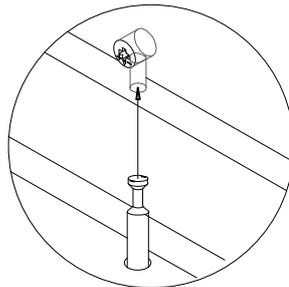
**STEP 2 - ALIGN THE CAM BOLT WITH THE HOLE AND PUSH TOGETHER UNTIL FLUSH. ( MAKE SURE THE ARROW OF CAM LOCK IS POINTING TOWARD THE HOLE ON EDGE OF PANEL. )**
