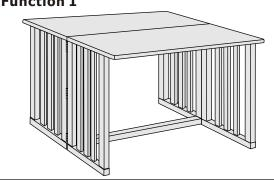
Attach the Table Top (1) to the Table Leg (2) and Frame Support (4) using JCBC screw (A), Spring Washer (C) & Flat Washer (D).
