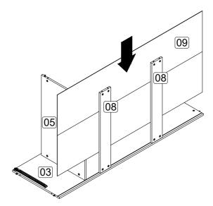
**Step 4:** Attach middle panel (5) and back bone (8) to side panel (4) using hardware A1 and A2 with a screwdriver (not provided).
