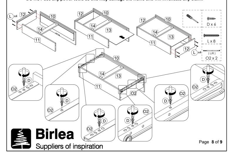
**Step 15:** Assemble the drawer in place along the drawer slides.
